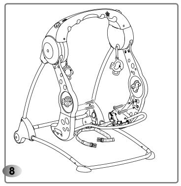
• Insert two #6 x 1.9 cm screws through each upper swing arm and into each lower swing arm. Tighten the screws.
